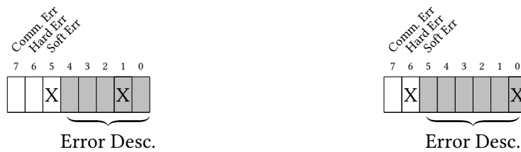
Figure 5.4: Two exemplary error status. Concretely, left byte field shows a recoverable error, indicating its refusal to a task. Right byte field represents a (non-recoverable) fault, indicating an aborted task on peer side.
