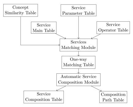
FIGURE 3.1: [44] SMA module diagram
