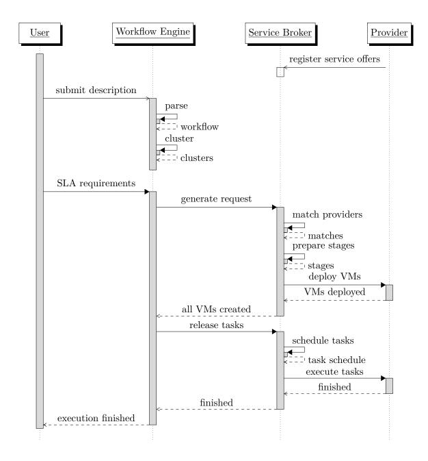
FIGURE 3.7: [14] workflow deployment sequence diagram
