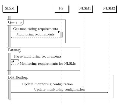
FIGURE 4.4: Monitoring requirements sequence diagram
