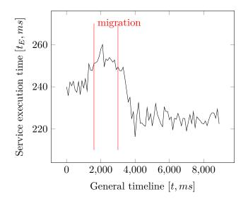
FIGURE 6.6: Composite service execution evaluation for network and processing ranking strategy
