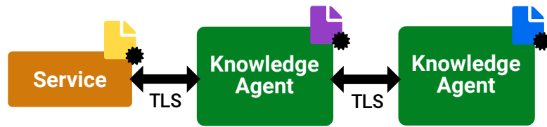
FIGURE 2.8: Authentication between a \mu -service and a KA (left) and between two KAs (right) to create TLS connections. Each entity uses a different certificate signed by the same CA.
