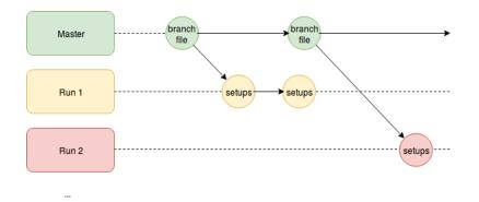
FIGURE 3.4: Structure of the Git repository used for distributing the setup files
