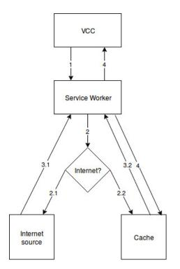
FIGURE 3.7: Procedure when the VCC requests data that is served by a Service Worker
