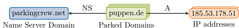
FIGURE 4.1: An exemplary setup of parked domains using name servers of ParkingCrew , resolving to ParkingCrew IP addresses.
