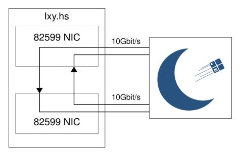
FIGURE 3.1: An illustration of the setup used to benchmark ixy.hs.
