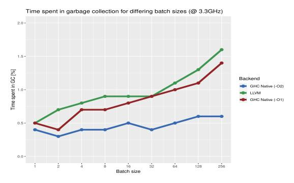
FIGURE 3.5: Time spent in GC for different backends and configurations.
