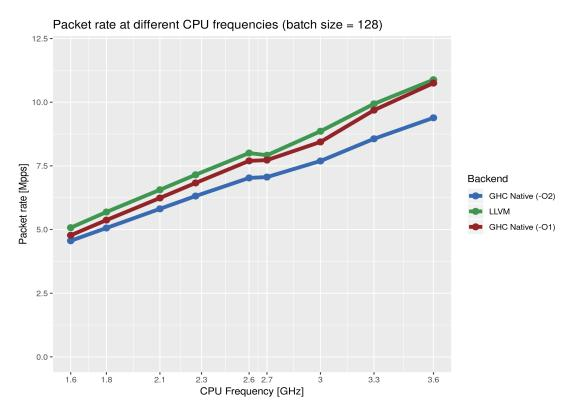
FIGURE 3.2: Packet rate vs. CPU frequency for different backends and configurations.
