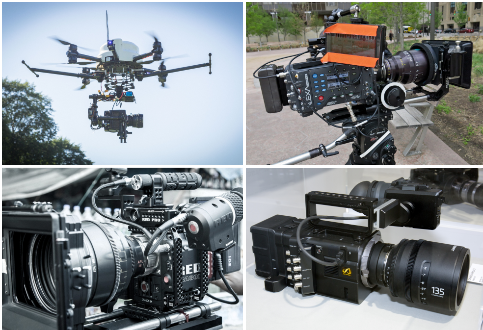
Figure 2.1: From top left, clockwise: ARRI ALEXA Mini (drone-mounted), ARRI ALEXA Plus, Sony PMW-F55 and RED Epic Dragon [3–6].
