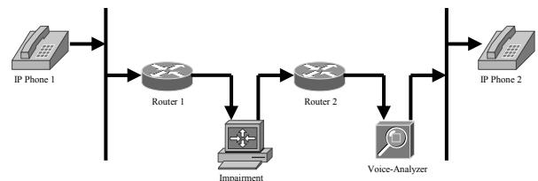
**Figure 7** Test environment for QoS measurements
