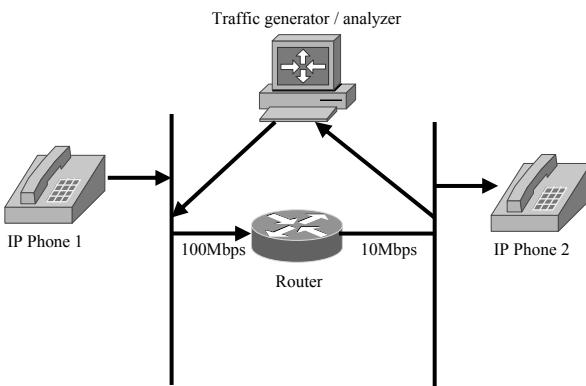
**Figure 8** Test environment for stress tests
