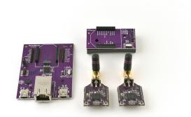
(OpenMote [2]) as well as open-source software should simplify the research in the area of cyber-phyical networks. The software implementation could be based on OpenWSN [3], which implements the required network stacks. An important requirement for the 6TiSCH implementation is the CoAP protocol [4]. CoAP is an HTTP-like protocol targeted to embedded devices and used e.g. for the 6TiSCH configuration.
