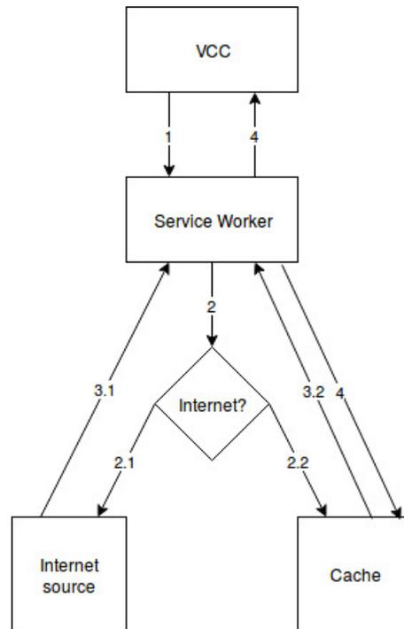
FIGURE 3.7: Procedure when the VCC requests data that is served by a Service Worker
