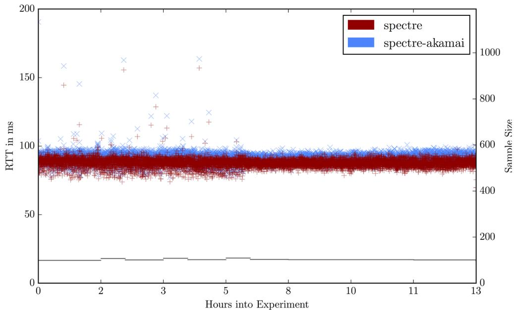
Figure 5.1: Scatter plot of httping-measured RTTs using HEAD requests
