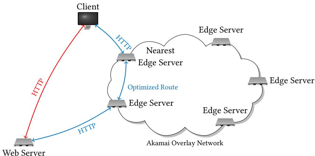
Figure 4.1: Illustration of using the nearest Akamai Edge Server for overlay network routing
