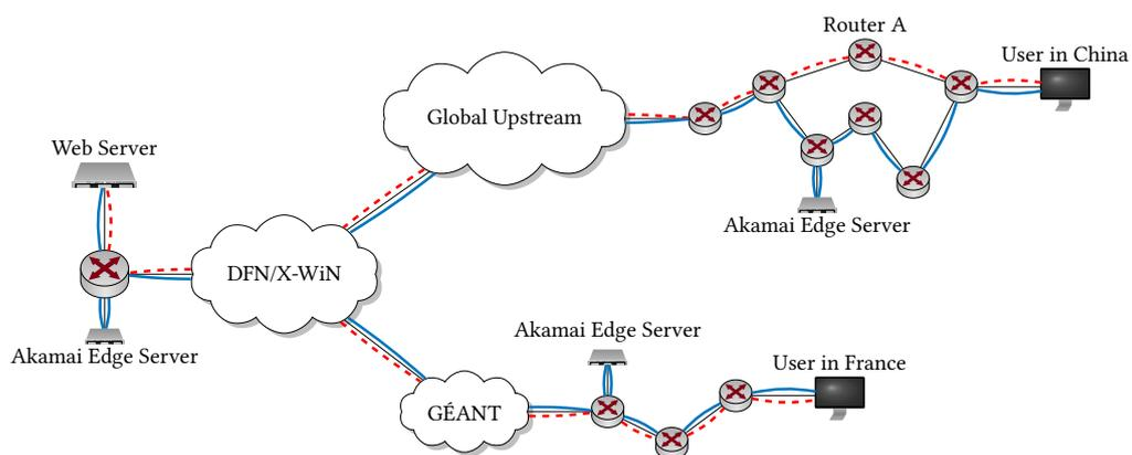
Figure 3.1: Example of diverging transport ways when using Akamai Overlay Network routing and plain Internet routing
