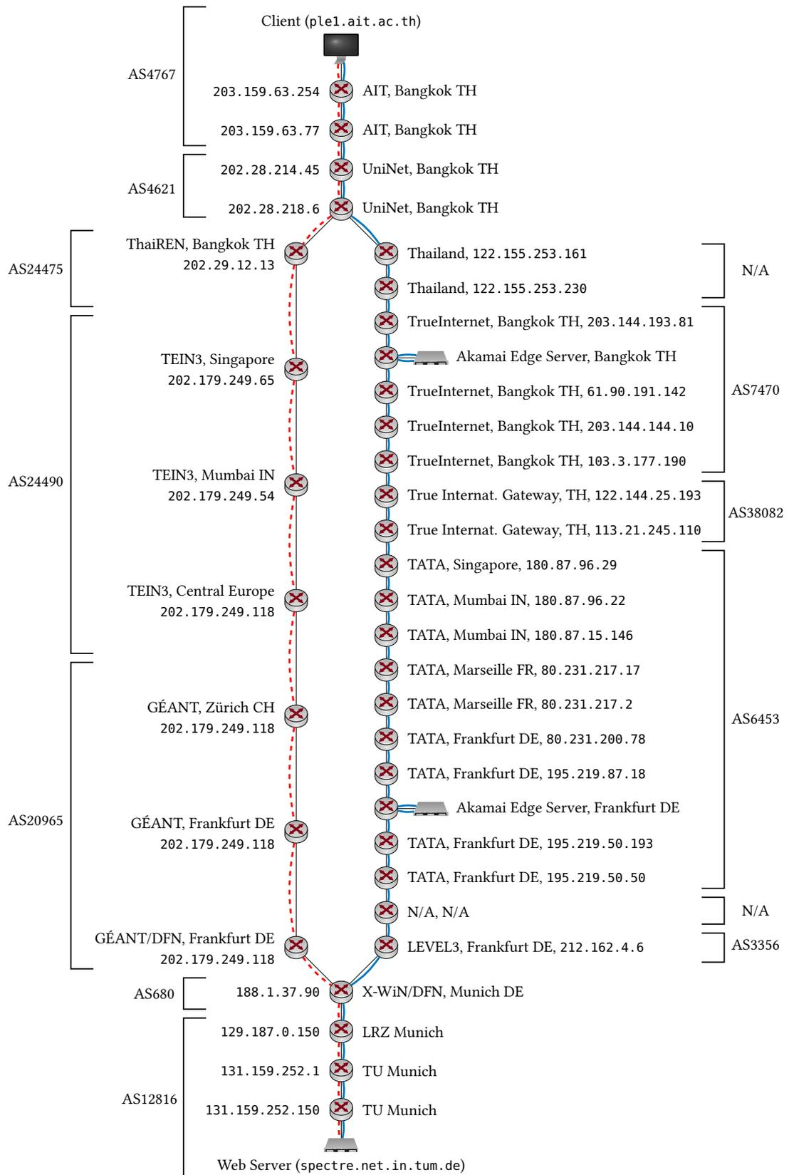
Figure 5.14: Graphical comparison of regular Internet and overlay network route from Bangkok to Munich
