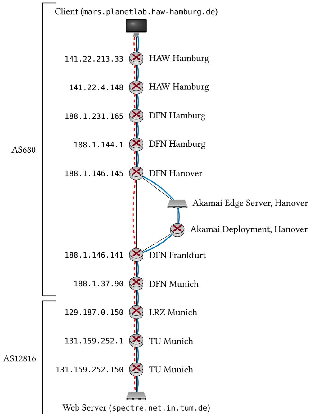
Figure 5.12: Graphical comparison of regular Internet and overlay network route from Hamburg to Munich
