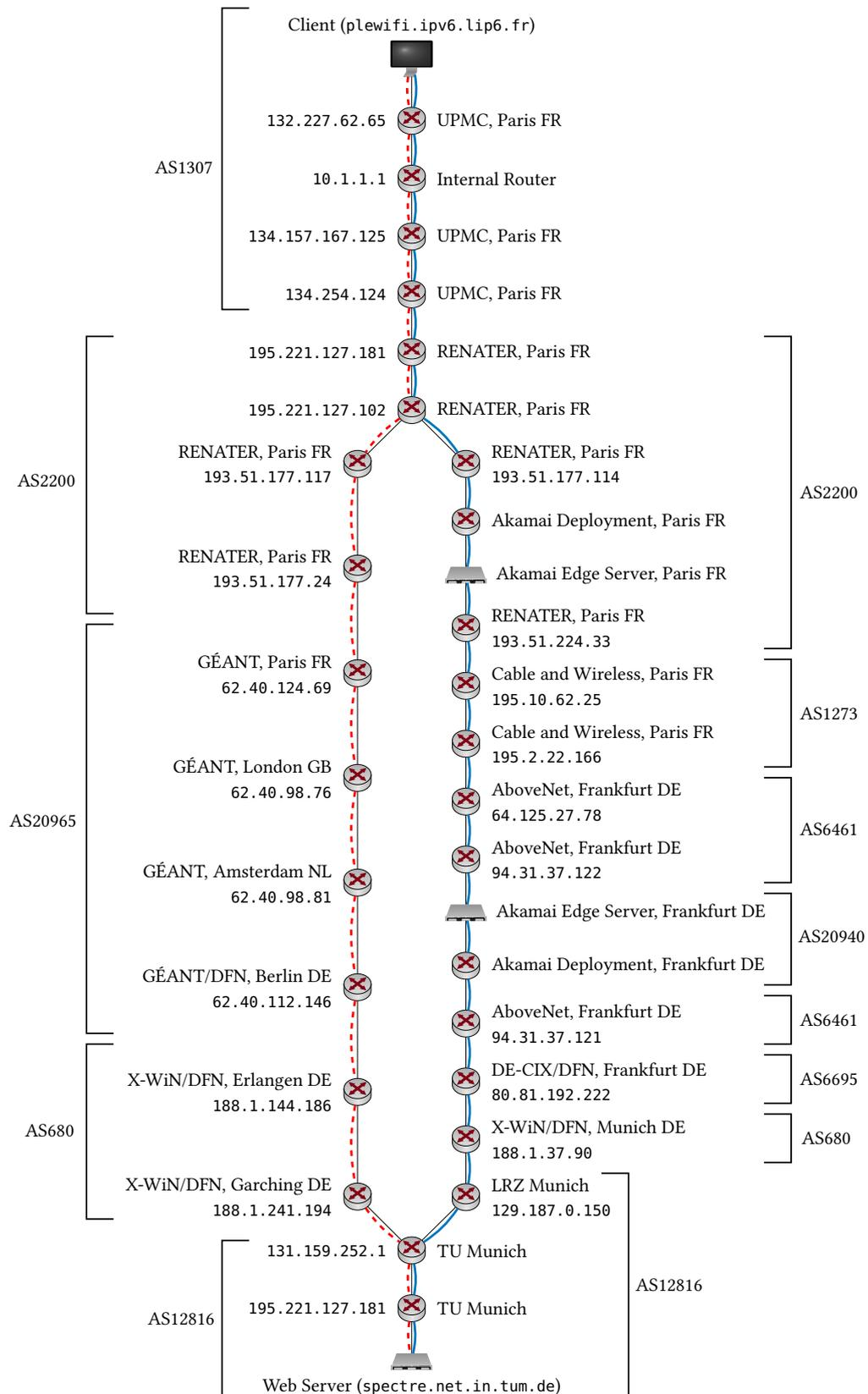
Figure 5.13: Graphical comparison of regular Internet and overlay network route from Paris to Munich
