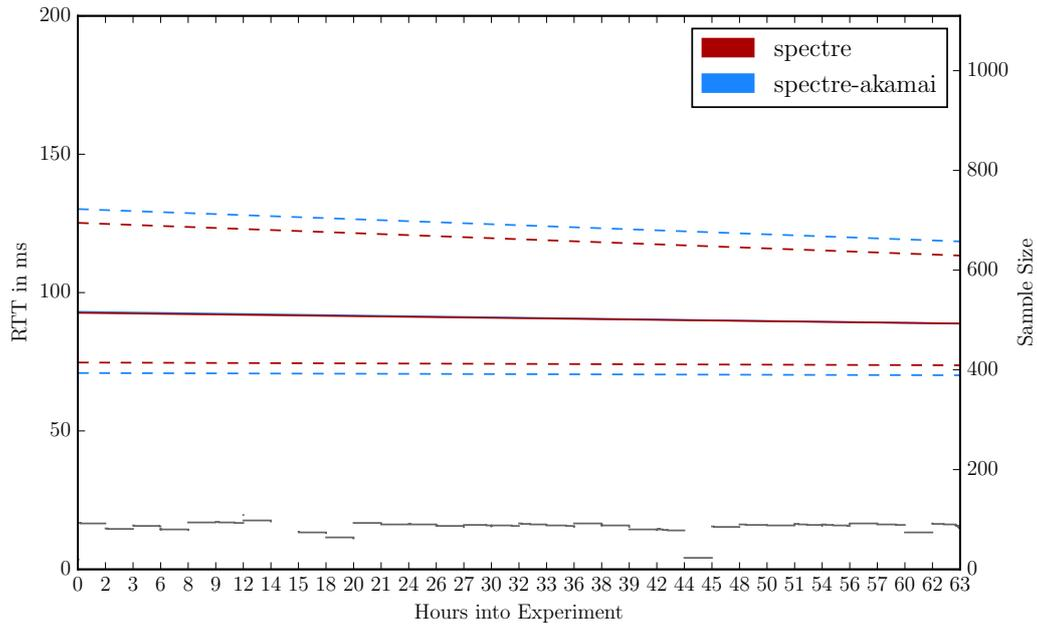
Figure 5.4: Linear regression plot of first quartile, median and second quartile RTTs measured by htping using GET requests
