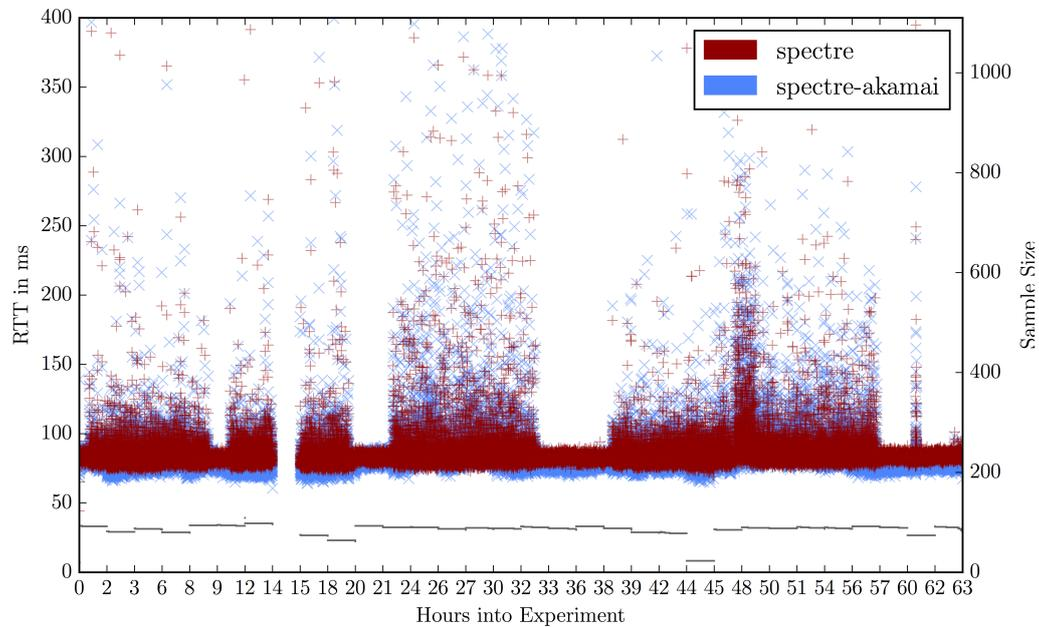
Figure 5.3: Scatter plot of httping-measured RTTs using GET requests
