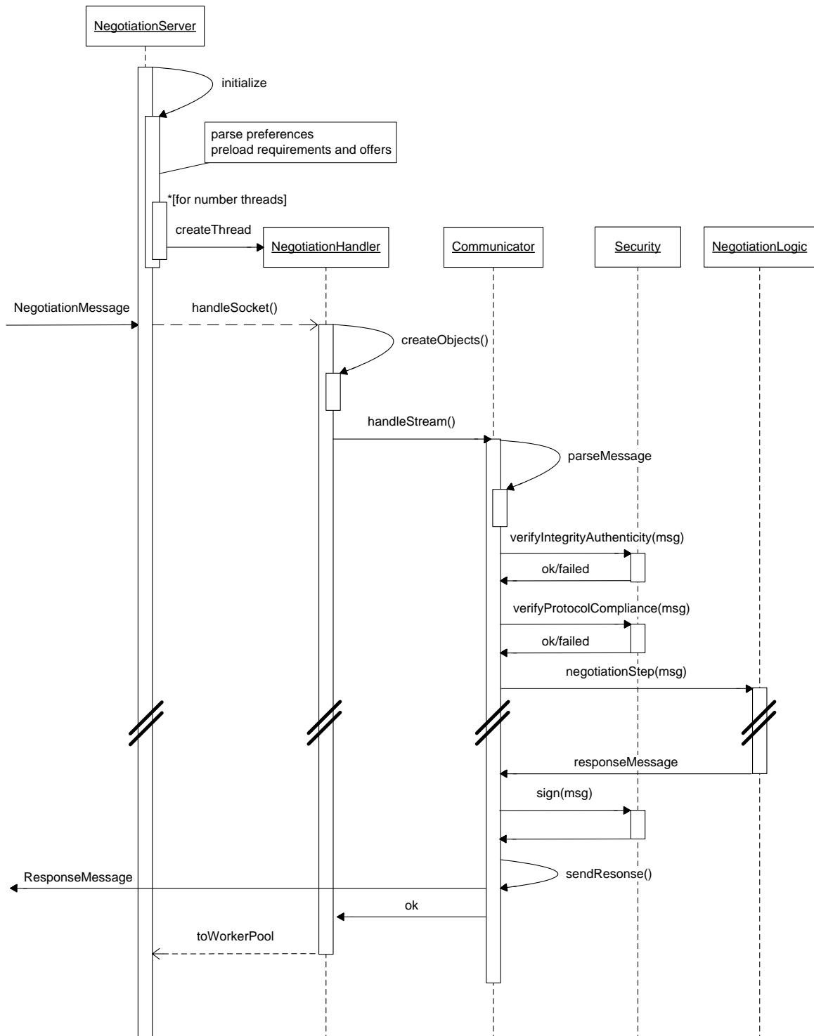
**Figure 7.6:** Time Sequence Diagram for handling Negotiation Messages at Server
