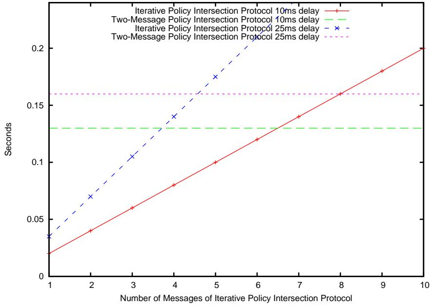
**Figure 4.8:** Time for Protocol Runs depending on Number of Messages for Iterative Policy Intersection Protocol and on Network Delay  $\sigma$
