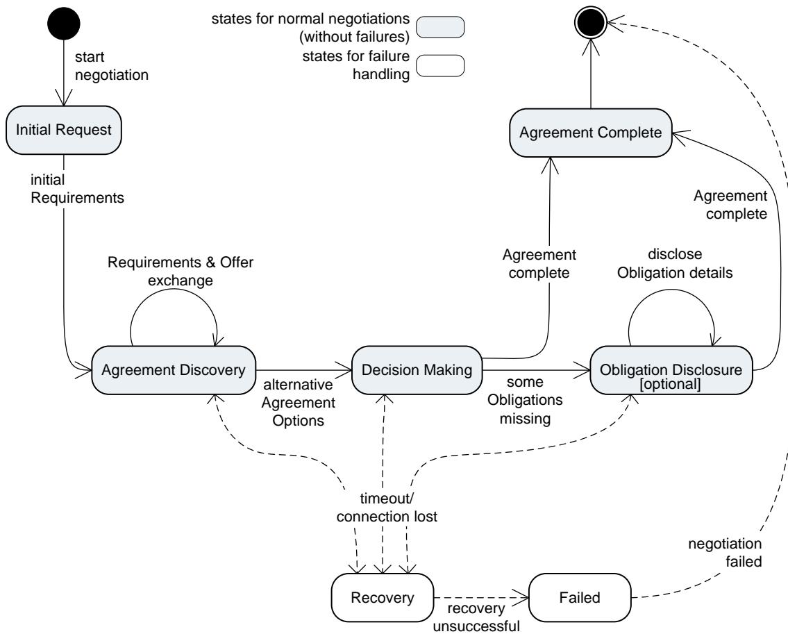
**Figure 5.5:** State Diagram of the Negotiation Process
