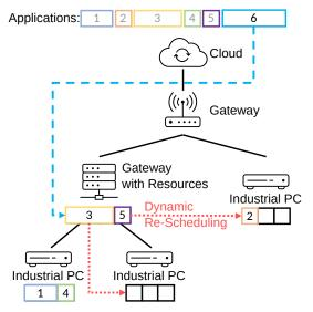
Since the topology and constraints of an IIoT network can change over time due to maintenance, hardware failure, hardware upgrades or expansion, a previously optimal solution may not satisfy the QoS constraint in the new network and we need to reschedule some or all applications dynamically at run-time.
