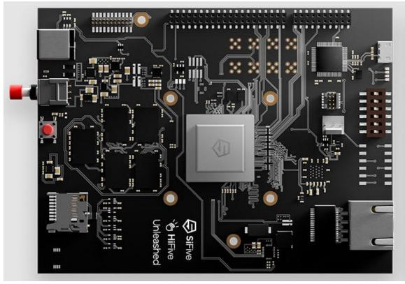
Play with an HiFive Unleashed dev board with a SiFive U540 64 Bit RISC V CPU and figure out how well it performs in various different scenarios.
