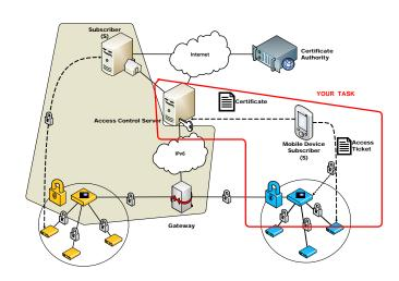
The implemented protocol should allow mobile devices to (1) interact with the sensor network directly and (2) allow access for the already collected data. In case (2) the mobile device can either access the data directly from WSN intern or from the global server where the data is stored. On the server site data banks must be implemented for the certificates and for the collected data. The protocol must be easy adaptable for new scenarios and devices. Finally the protocol must be evaluated.
