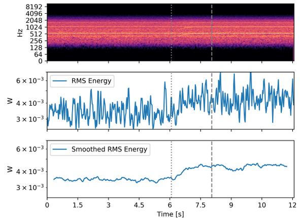
Fig. 2. A server spinning up its fans during boot. The top part shows the log power spectrogram of the filtered signal. The middle plot shows the RMS energy for the spectrogram. The bottom plot shows the smoothed RMS energy. The dotted and dashed line mark start and end of the identified event.
