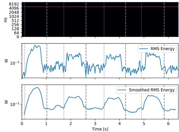
Fig. 4. Error code emitted by a server’s buzzer due to a faulty fan
