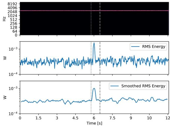
Fig. 3. Detection of a short single-frequency event in our first experiment
