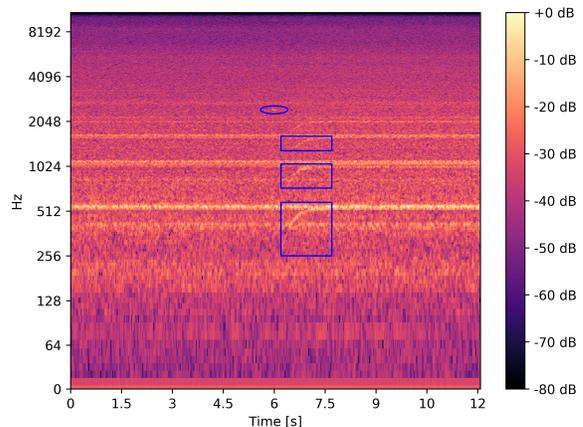
Fig. 1. Log power spectrogram of a recording in our DC. The ellipsis marks a beep that is emitted by a booting server. The rectangles mark the fans of a server spinning up during its startup.
