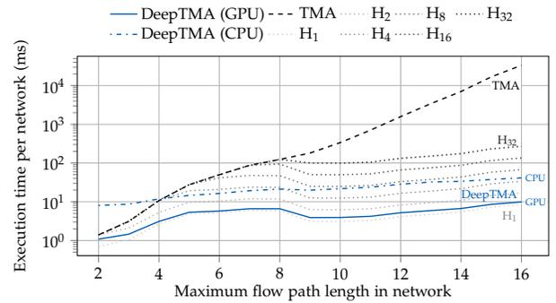
Figure 15: Execution times per topology for TMA, DeepTMA and  $H_n$  heuristics on the dataset from [11].
