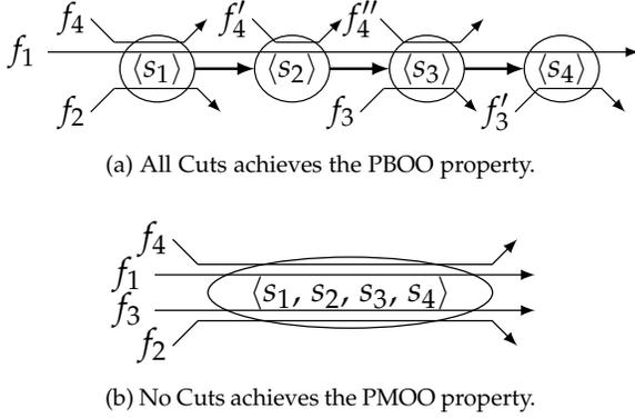
Figure 3: Reduction rules in the NC analysis.
