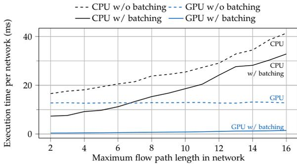
Figure 14: Execution time of the cut recommendation part of DeepTMA, executed on CPU or GPU, without batching or batch sizes of 64 networks on the dataset from [11].
