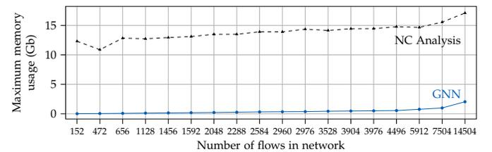
Figure 16: Memory usage of the GNN and the TMA NC analysis on the dataset from [11].
