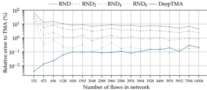
Figure 11: Relative error of DeepTMA on the dataset from [19] with much larger networks.
