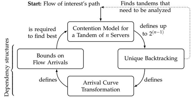
Figure 7: Dependency cycle defining current NC analyses.
