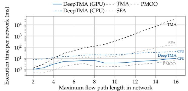
Figure 13: Comparing DeepTMA to existing NC heuristics on the dataset from [11].
