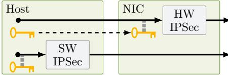
Figure 2. NIC accelerated and software IPsec processing path
