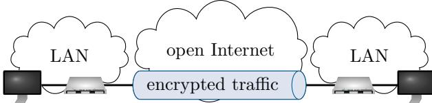
Figure 1. IPsec VPN tunnel mode
