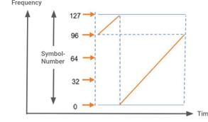
Figure 2: cyclically shifted up-chirp of symbol 96, Adapted from: [3]
