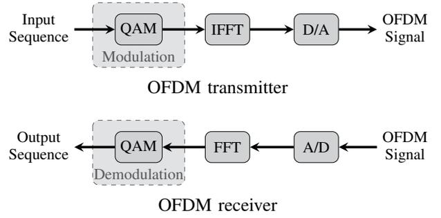
Figure 2: OFDM system based on [8], [10].
