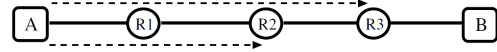
Figure 4: Building Blocks: The properties of link R2 \rightarrow R3 can be estimated by subtracting the measured properties of path A \rightarrow R2 from the measured properties of path A \rightarrow R3 . [2]
