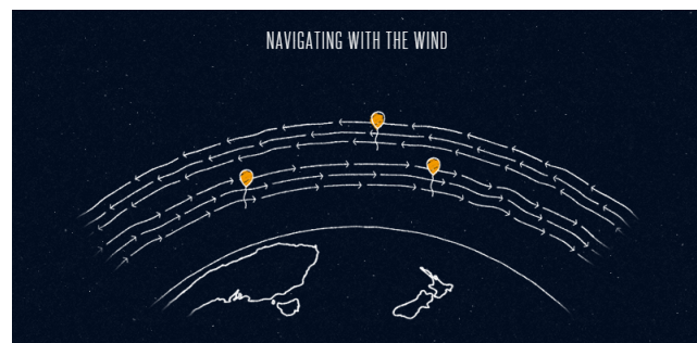
Figure 2: Project Loon utilizes the properties of stratified winds in the stratosphere.[9]
