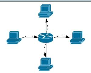
send\_packet\_out tells a switch (argument 1) to send out a packet
