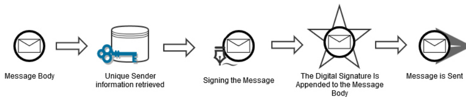
Figure 2.3: The process of digitally signing a message
