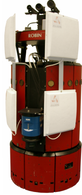
Figure 9 Experimental platform: An RWI B21 mobile robot with an UHF RFID reader by Alien Technology, two pairs of RFID antennas (white), and a laser range finder (blue, mounted in front of the robot) for reference localization. The WLAN and Bluetooth antennas are mounted on top of the robot.
