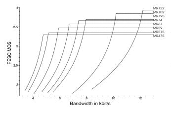
Figure 6: MOS vs. bandwidth and coding rate (MR475=4.75kbps, MR122=12.2kbps).
