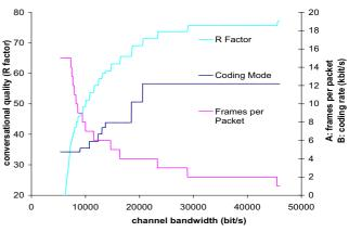
Figure 7: Choosing optimal coding rate and packetization on packet-switched link.
