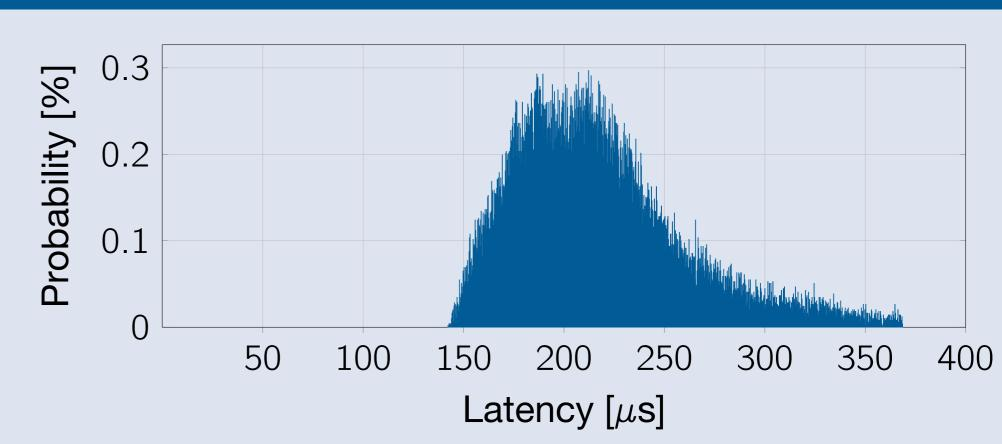
Latency distribution of traffic forwarded through a VM running on top of Open vSwitch at a load of 322k packets/s.
