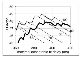
Figure 3 Zoom view of figure 2: Fixed, adaptive and no-deadline scheduling (normal, dashed, and bold line respectively)
