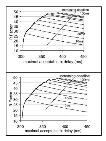
Figure 2 Telephone quality vs. maximal acceptable transmission delay using adaptive (top) and fixed scheduling (bottom) with different deadlines
