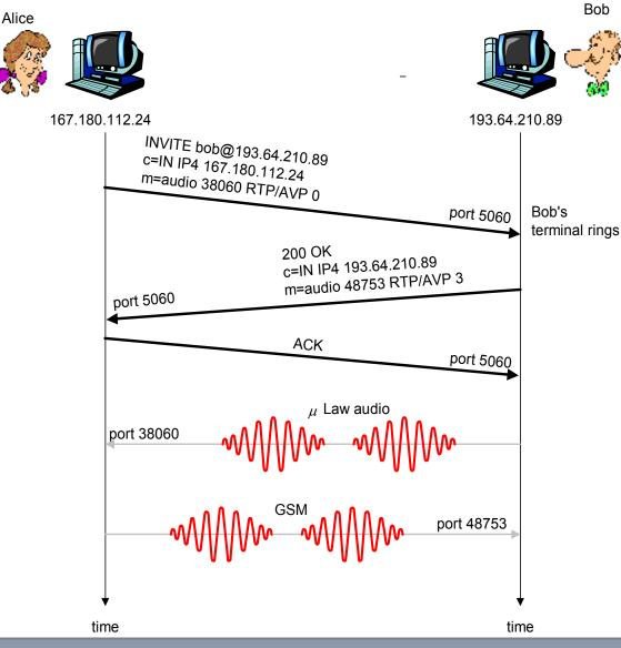
□ Alice's SIP invite message indicates her port number, IP address, encoding she prefers to receive (e.g. AVP 0: PCM ulaw) Bob's 200 OK message indicates his port number, IP address, preferred encoding (e.g. AVP 3: GSM) SIP is an out-of-band signalling protocol □ SIP messages can be sent over TCP or UDP. (All messages are ack'ed) □ default SIP port number is 5060 for TCP and UDP, and 5061 for TSL-over-TCP.
