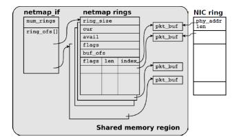
Figure 8: The structures of the netmap architecture (image from [12])
