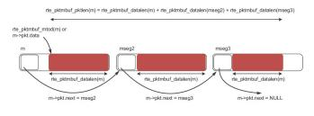
Figure 7: One packet as chain of  $rte\_mbuf$ s. Every  $rte\_mbuf$  contains the same metadata, a pointer to the next buffer and a part of the packet data (image from [8])
