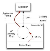
Figure 10: PF\_RING Direct NIC Access driver (image from [14])
