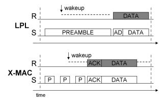
Figure 6: Difference between standard LPL and X-MAC protocol
