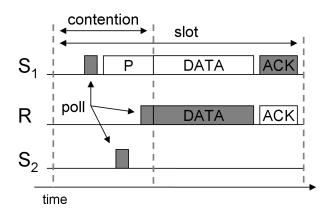
Figure 5: Crankshaft contention and message reception
