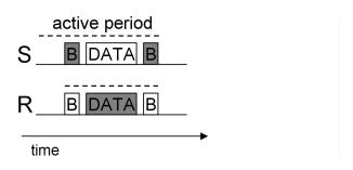
Figure 7: RI-MAC: Initiation of data exchange by the receiver R
