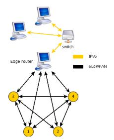
Figure 11: 6LowPAN network integrated into IPv6 network
