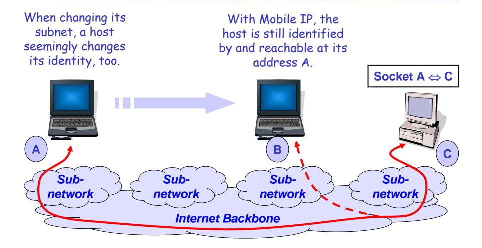
Mobile IP occupies a different point in the design space than DynDNS. It keeps the double role of IP addresses as locator and identifier.
