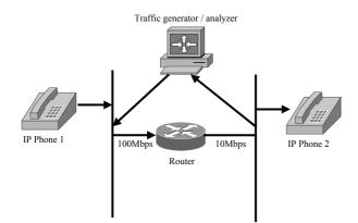
Figure 8 Test environment for stress tests
